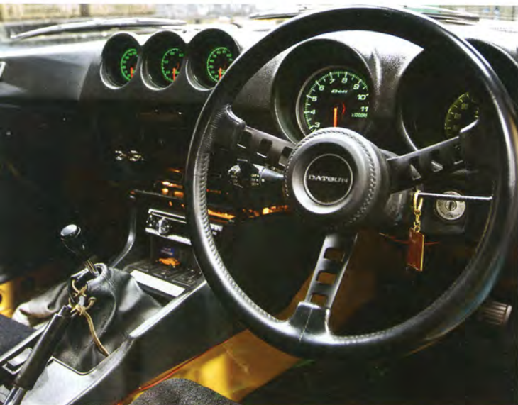
DEFI gauges, including an 80mm tachometer, fit perfectly in the holes and put a modern twist on a classic dash.
